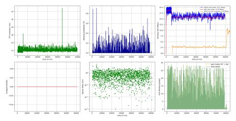
Standard behavior of the L4S architecture with one LL and one classic flows. Horizontal axis is the time in ms.
