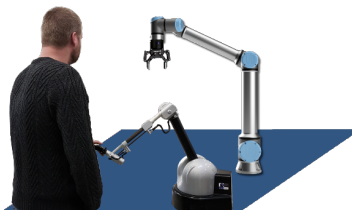
Figure 11: Example of haptic device, the 1to1Teleroobotics extender from Haption and Universal Robotics
